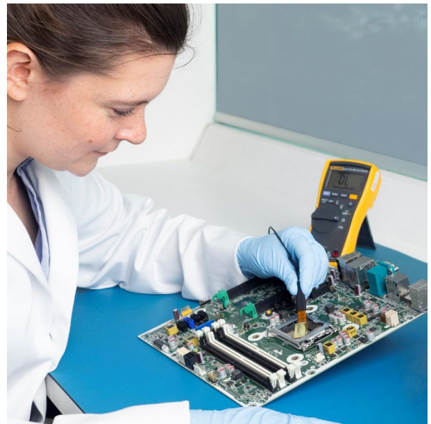
Figure 8 Model FHF05-15X30 with GLD-15X30 being installed to measure heat flux on a computer processor. The sensor is mounted on a well-prepared flat surface.
