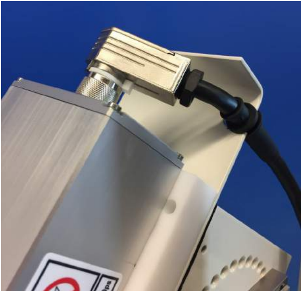
Figure 13: Mounting the connection cable to the sensor. The protective rubber sleeve is inserted into the recess of the floor plate during cable mounting. The amphenol connector can be adjusted to the angle (45° steps) when the white mounting ring is released.
