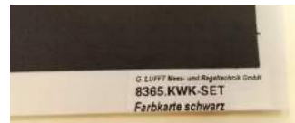
Figure 9: target plate set consists of a white and black calibrated plate for reference measurements in field and lab
