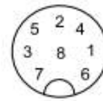
Figure 17: View on soldering connection of the cable box with notch.
