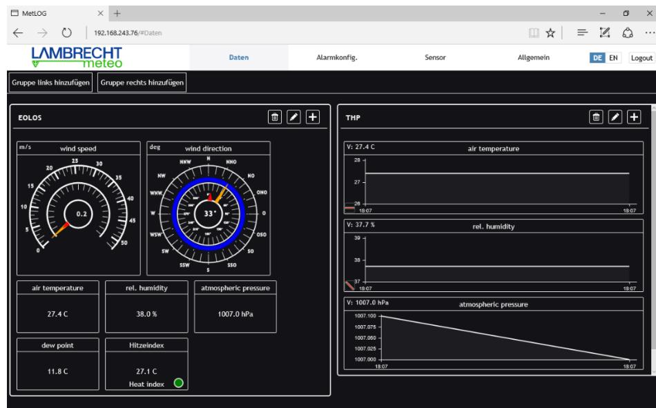
The met[LOG] is a small serial 3.4 channel data logger with 3 serial interfaces, 4 analogue/digital interfaces and connection to LAN (Ethernet). The met[LOG] has an integrated web server, which allows for calling and displaying data directly via a browser. Warnings and alarms can be called via the 4 digital outputs.
