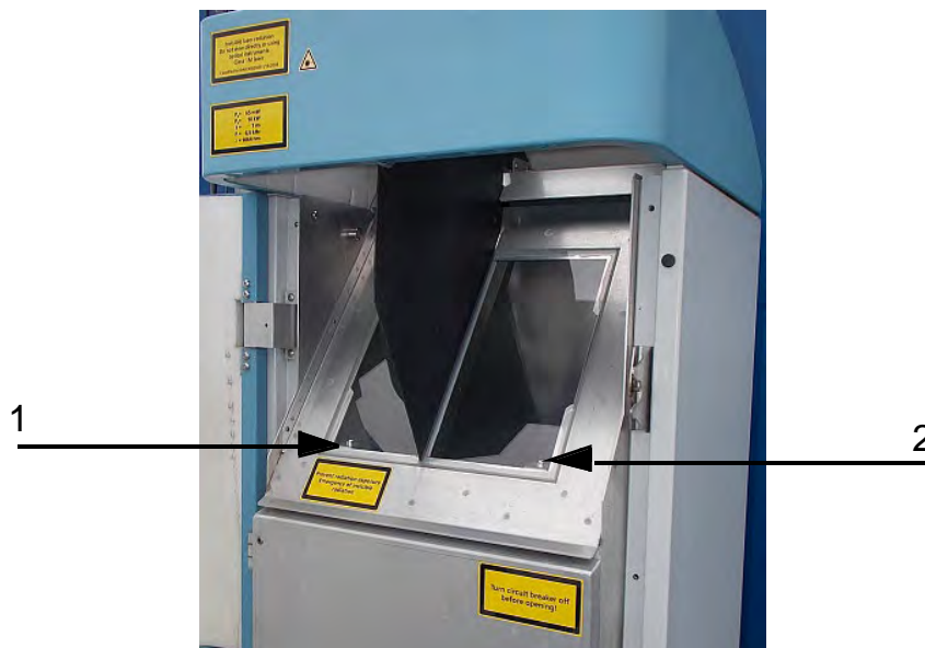
Figure 32 Windows to be cleaned.
