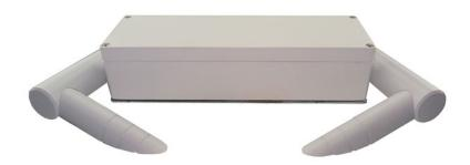
New product version of the known Lufft VS20 visibility sensor with a measurement range of 10...2000m, easy calibration functionality, sea waterproof housing and (active) spider defence
