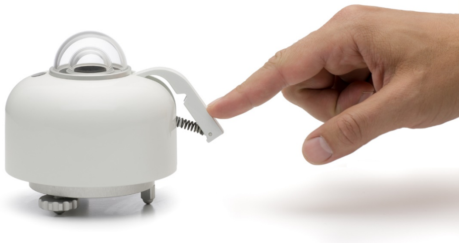
Figure 4.2.2 Installation of 16131.5's sun screen
